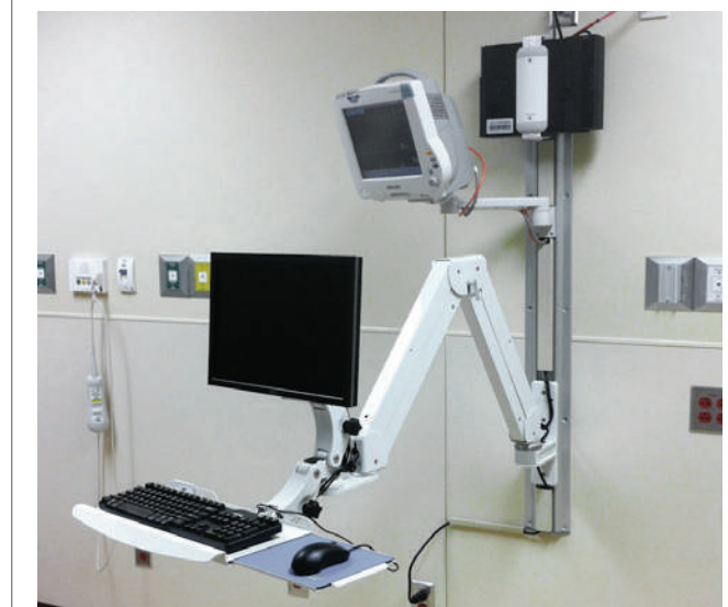
Placement of medical device on ICW track
